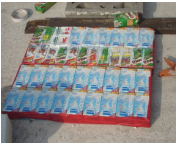
Figure 3. The panel of used milk containers filled with rice husk.
