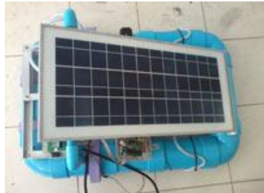
Figure 5. The power supply using a solar cell.
