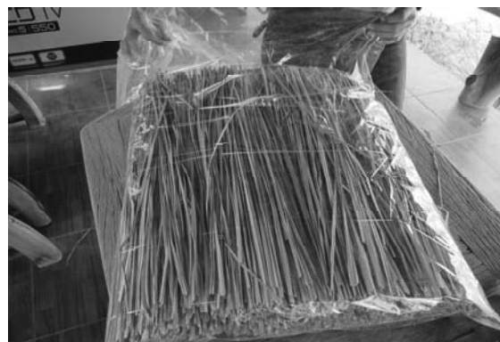
Figure 4. The plastic bags and silica gel were used to cover the grass to protect insulation from moisture and insects.
