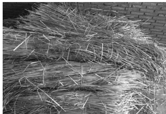
Figure 3. The physical character of sun-dried 'Vetiver Grass' that used to make local thermal insulation.
